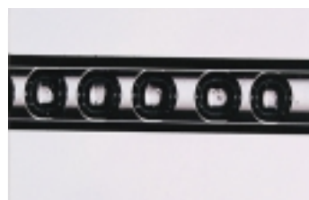
Fig. 2: Image of a micro-capillary lens taken with an optical microscope. The inner diameter of the glass capillary is 0.8 mm.
