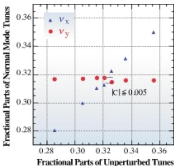
Figure 2: Tune separation for resonance difference; the resonance width ( $|k|$ ) is about 0.005.
