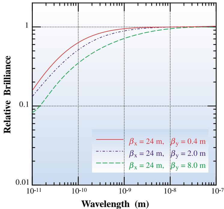
Figure 6: Relative brilliance as a function of wavelength for three different  $\beta_y$  at ID section:  $\beta_y = 8.0$  m in normal operation and  $\beta_y = 0.4$  m with optimization of brilliance to maximum value.
