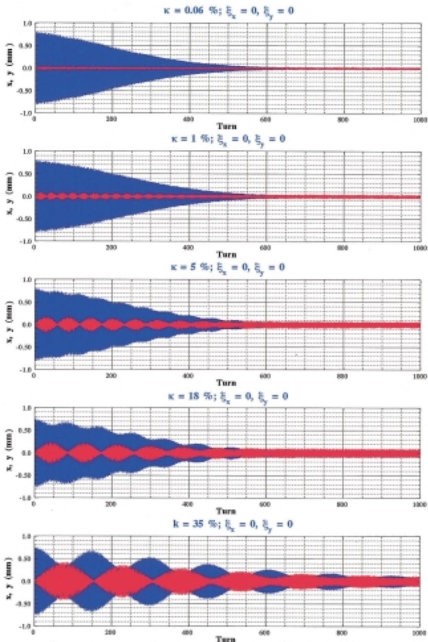
Figure 3: Horizontal (blue) and vertical (red) coherent oscillations measured after a horizontal kick.
