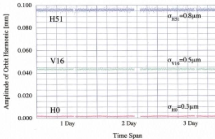
Figure 5: Amplitude changes of tune harmonics (51st for horizontal (blue) and 16th for vertical (green)) and 0th harmonic (circumference change (red)) in COD for three days with periodic correction of global orbit.
