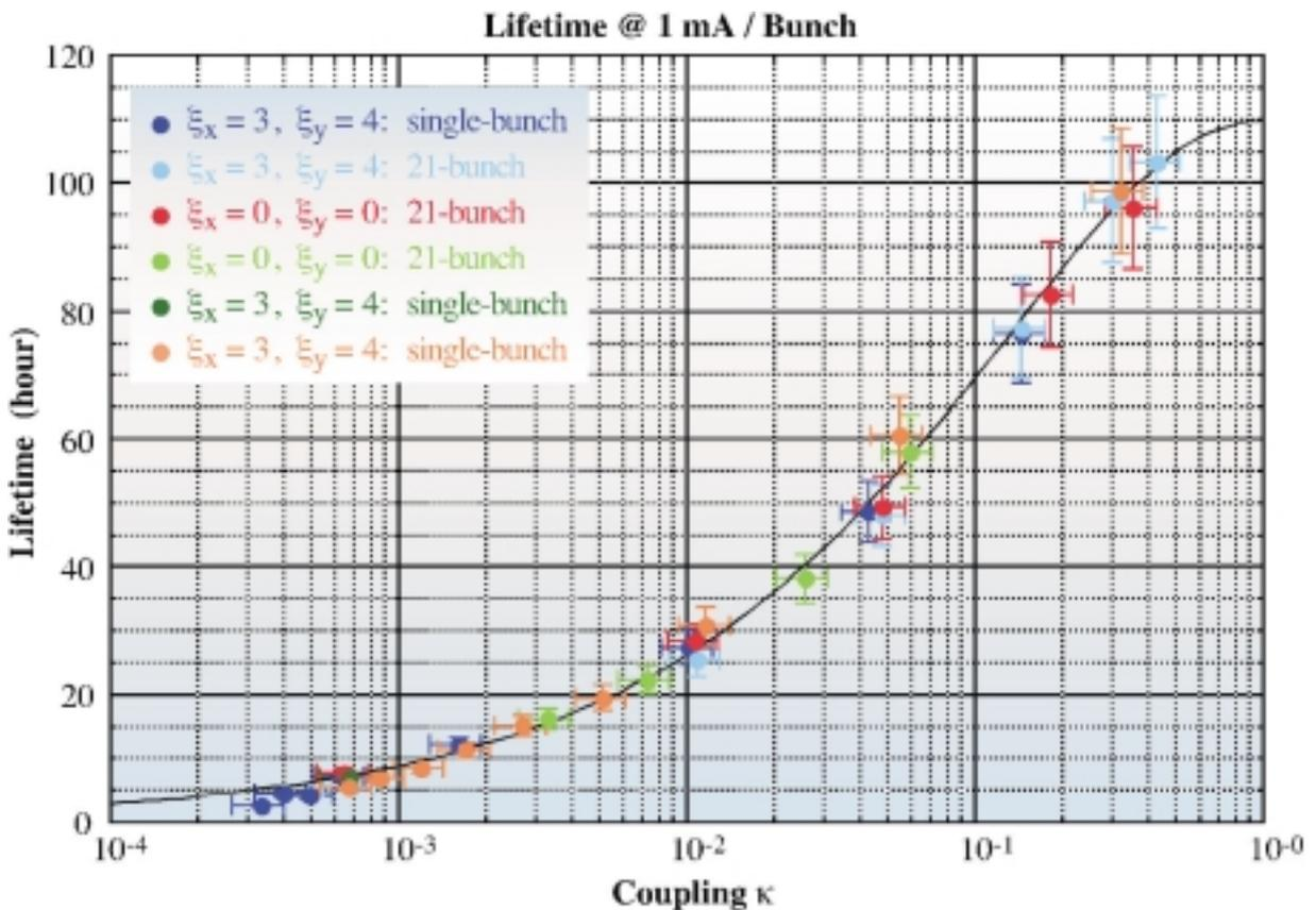
Figure 4: Beam lifetime as a function of betatron coupling ( $\kappa$ ); solid line shows the theoretical Touscheck lifetime.
