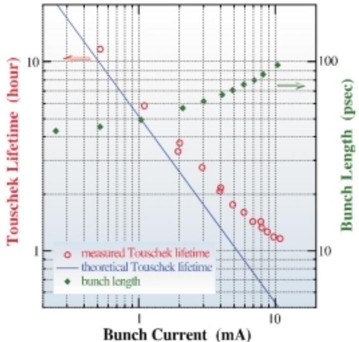
Figure 1: Beam lifetime and bunch lengthening as a function of bunch current.
