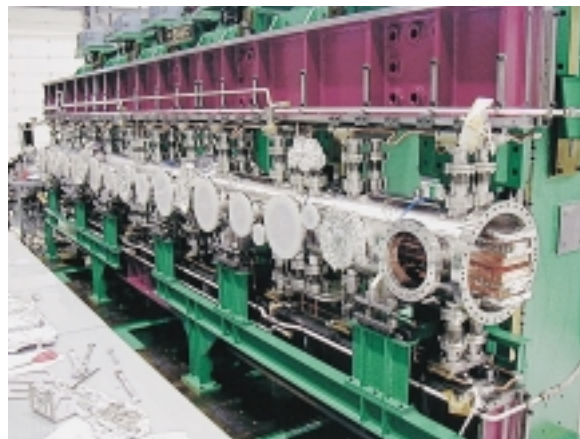
Figure 1: Photograph of in-vacuum undulator; ion and NEG pumps are not attached yet.
