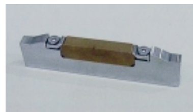
Figure 2: One magnet unit of the in-vacuum undulator; four magnet units form one period.
