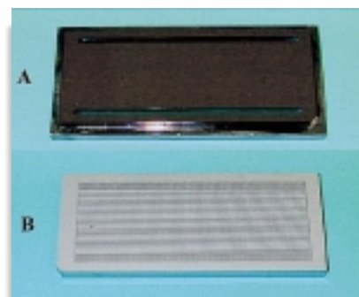
Figure 3: Improved-design pinpost crystal: (A) water distributor (bonded side), (B) top plate with pins before mechano-chemical polishing.
