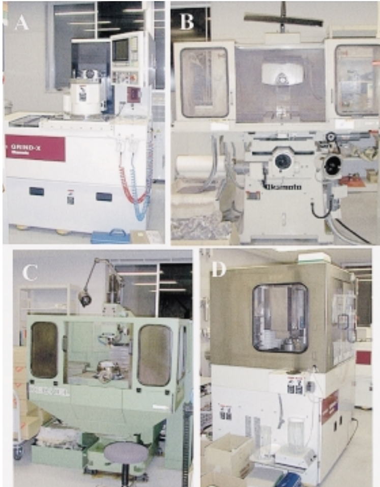
Figure 4: Crystal fabrication facilities at SPring-8: (A) grinder, (B) diamond cutter, (C) diamond milling machine and (D) mechano-chemical polisher.
