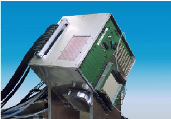
*Fig. 1. Photograph of Micro-Strip Gas Chamber mounted on a mother board with anode- and back-strip preamplifier boards.*
