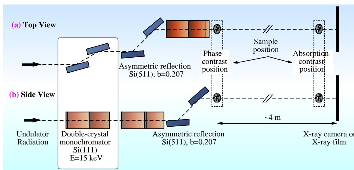
Fig. 1. Optical system for phase-contrast X-ray imaging. (a) Top view and (b) Side view. The original beam size is expanded by using asymmetric Bragg reflection in both vertical and horizontal directions. Absorption-contrast imaging can also be performed simply by placing the sample just in front of the image sensor.
