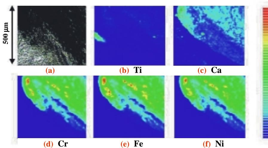
Fig. 2. (a) Optical microscopic photograph of the tissues around a failed hip replacement prosthesis. (b-f) Elemental maps of (b) Ti, (c) Ca, (d) Cr, (e) Fe and (f) Ni. The scanning area was 500 μm<sup>2</sup>. All images are 50 × 50 pixels of 10 μm resolution and the measurement time was 1 sec/pixel. The scale on the right-hand side of the images shows the count of the X-ray intensity. The range of intensity is 84 for Ca, 210 for Ti, 3300 for Fe and 490 for Ni.
