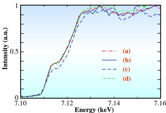
Fig. 3. Fe K-edge XANES spectra measured at point (a), (b), (c) and (d) in Fig. 1(a).
