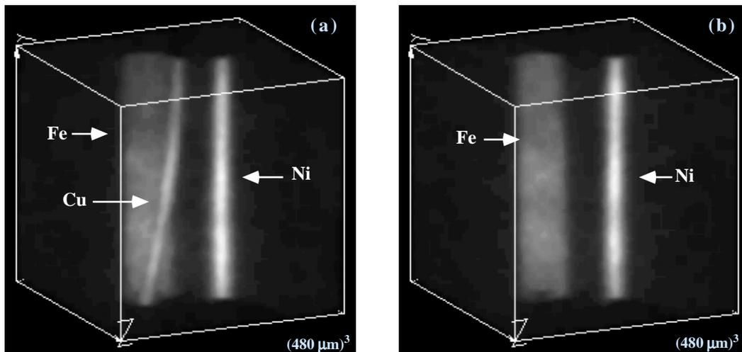
Fig. 2. 3-D reconstructed images of Cu, Ni and Fe wires at the excitation X-ray energy of (a) 9.00 keV and (b) 8.43 keV. The  $(480 \mu\text{m})^3$  cubic volume is shown. The images were reconstructed from 50 X-ray images from different angles of view with the same interval of 7.2 degrees. The exposure time of each X-ray image was 60 s.
