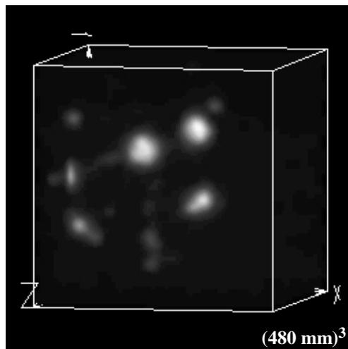
Fig. 3. 3-D reconstructed image of a synthetic diamond at an excitation X-ray energy of 8.34 keV. The images was reconstructed from 50 X-ray images from different angles of view with the same interval of 7.2 degrees. The exposure time of each X-ray image was 8 min.
