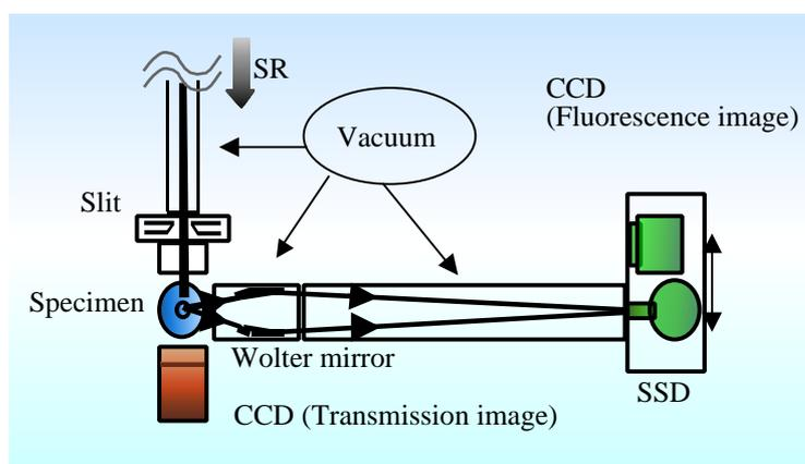
Fig. 1. Optical arrangement of the X-ray fluorescence microscope.
