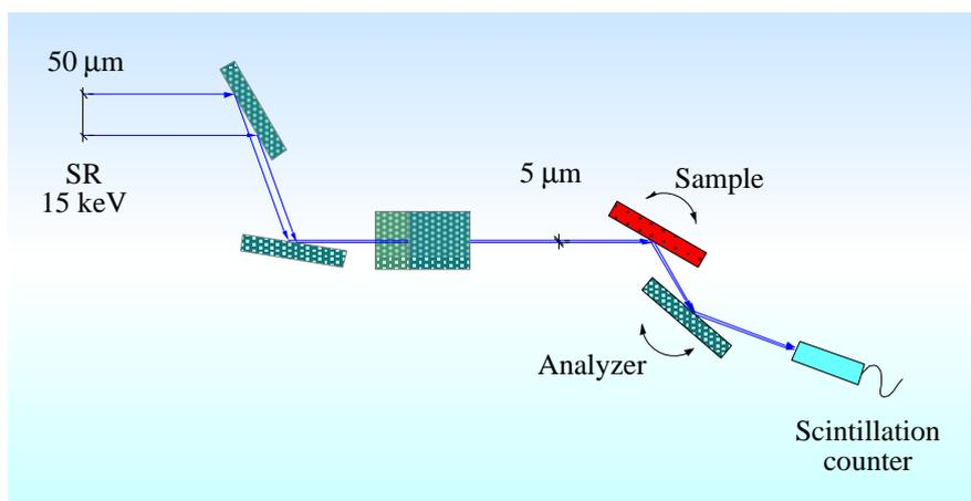
*Fig. 1. Optical system for parallel X-ray microbeam experiments. The X-ray beam was compressed and collimated by adopting 115 (+, -) successive asymmetric reflections from Si (001)-surface crystals in both horizontal and vertical directions. The analyzer crystal is removed from the X-ray path in the rocking curve measurements.*
