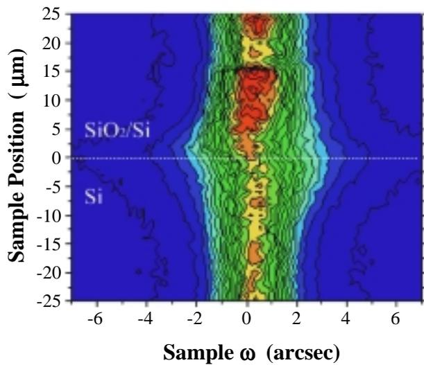
Fig. 2. The results of the rocking curve measurements. The contour map represents the diffraction intensity. The vertical axis gives the sample position. The Si area is in the negative position and the SiO<sub>2</sub>/Si area is in the positive position.
