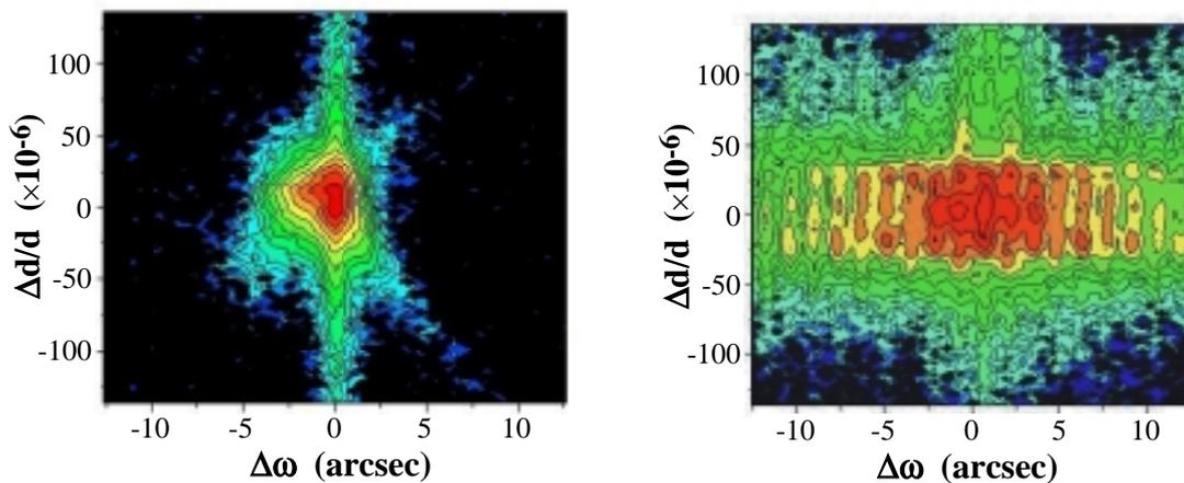
Fig. 3. 004 reflection reciprocal lattice maps. (a) the Si area and (b) the minute oxidation pattern region.
