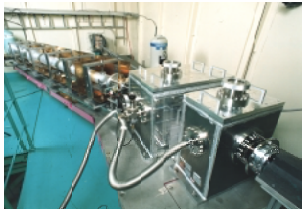
Fig. 2. Cauchois-type analyzer assembly, consisting of three separate triangle bent-crystals of Si 620 with 1 mm thickness.
