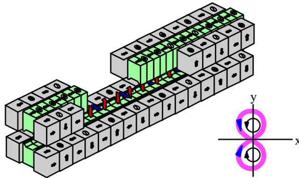
Fig. 4. Magnet design of the in-vacuum figure-8 undulator.
