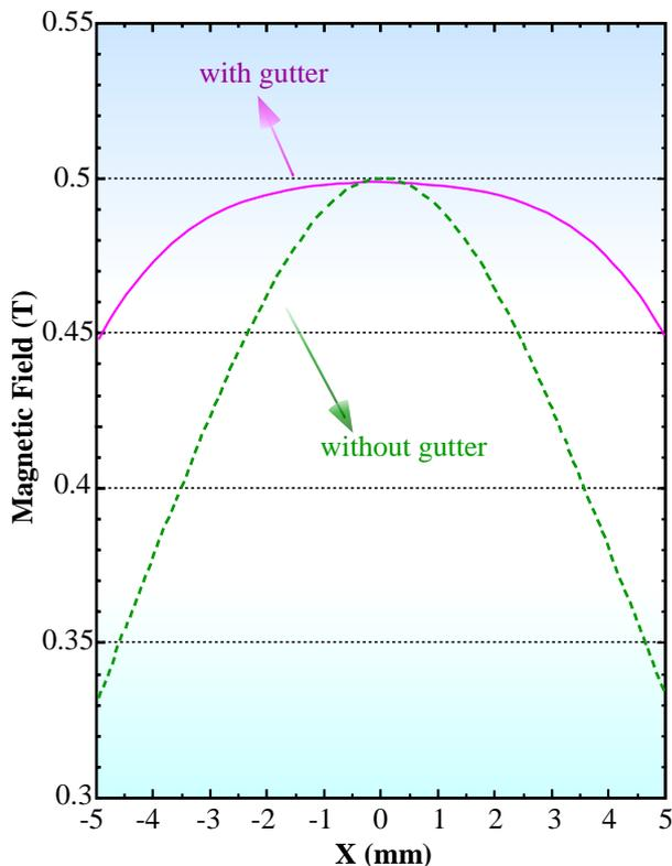
*Fig. 3. Comparison of calculated field uniformity using an in-vacuum vertical undulator with and without gutter.*
