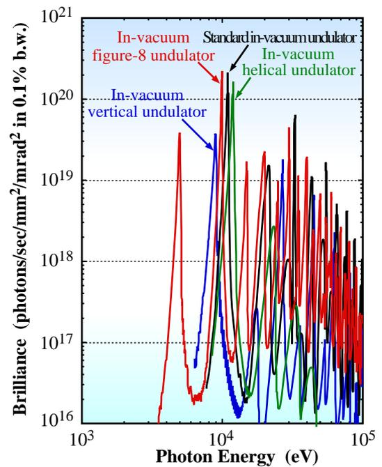
*Fig. 1. Spectral brilliances obtained from the in-vacuum undulators of exotic type, an in-vacuum vertical undulator, an in-vacuum figure-8 undulator and an in-vacuum helical undulator. For comparison, a spectrum from a standard in-vacuum undulator is also shown.*
