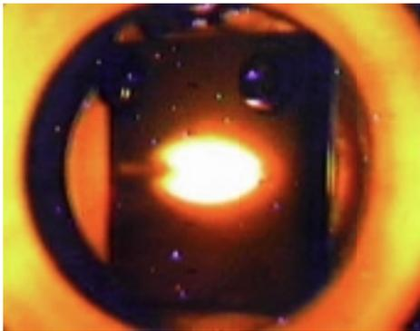
Fig. 5. Image of the radiation obtained from the in-vacuum figure-8 undulator.
