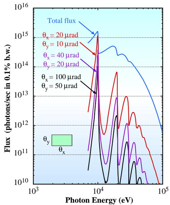
Fig. 6. Spectral flux of the in-vacuum helical undulator calculated for various aperture values of the spatial filter.
