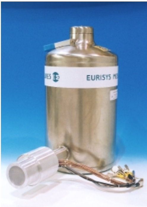
Fig. 2. Prototype microstrip germanium detector with a strip pitch of 350 \mu\text{m} .
