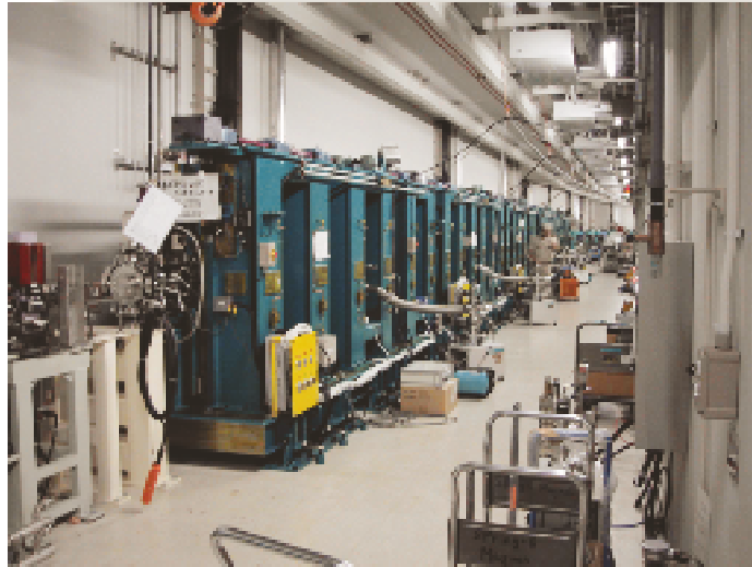
Fig. 3. 27 m in-vacuum undulator installed in the SPring-8 storage ring.
