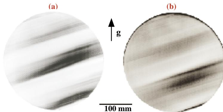
Fig. 3. X-ray topographs of a 300-mm-diameter CZ silicon crystal after slicing, followed by slight etching. (a) and (b) were taken using the asymmetric 511 reflection of 21 keV X-rays at the low-angle side and the high-angle side of the rocking curve, respectively. The arrow designates the diffraction vector *g*.
