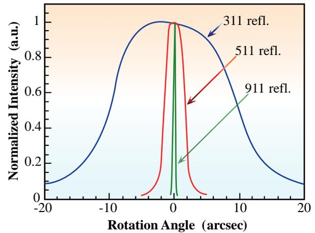
Fig. 2. Calculated rocking curves from (100) silicon. Incident angle was fixed at 1 degree; the asymmetric 311, 511 and 911 reflections used 8.7, 21 and 60 keV X-rays, respectively.
