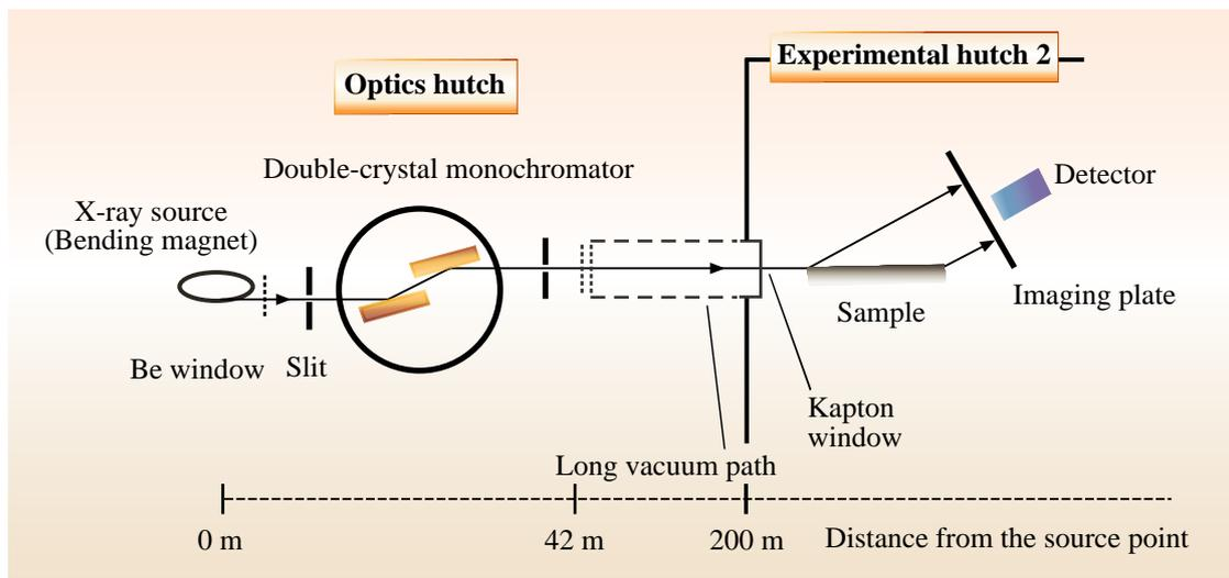
*Fig. 1. Schematic diagram of the optical system for large-area X-ray diffraction topography. The 300 mm- wide and monochromatic X-ray beam, obtained at the 200 m point apart from the bending-magnet source, was used to acquire topographs of a 300-mm-diameter silicon crystal sample.*
