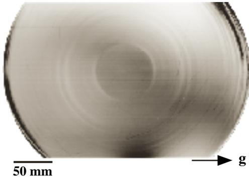
*Fig. 4. X-ray topograph taken with the asymmetric 12 2 2 reflection of 60 keV X-rays after a polishing test. Circular patterns were identified as surface damage caused by polishing. The arrow designates the diffraction vector  $g$ .*
