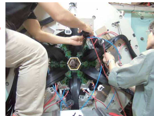
Fig. 2. Charged particle detector and its adjustment.
