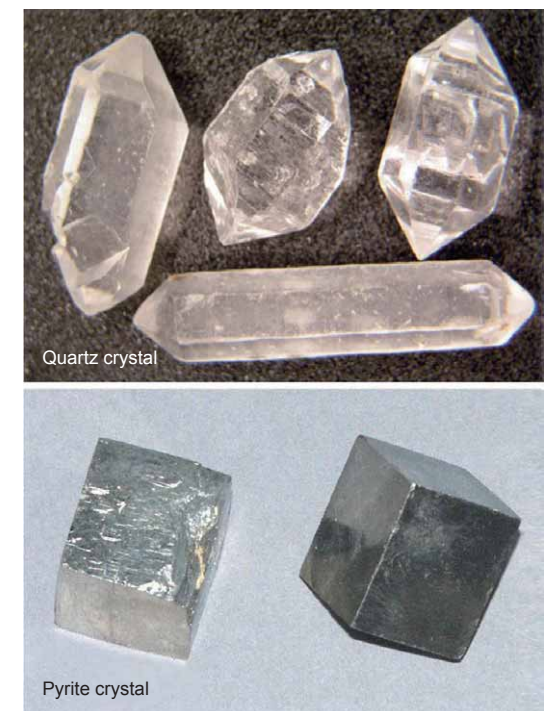
Fig. 3. Quartz crystal and pyrite crystal. Quartz crystals are hexagonal cylinder-shaped, whereas pyrite crystals are dice-shaped.
