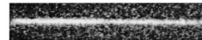
Fig. 1(a). Luminous image observed with the X-ray beam at 12 keV, corresponding to the photoelectron energy of 8.8 keV. The range of the photoelectrons was estimated to be 1.1 mm.
