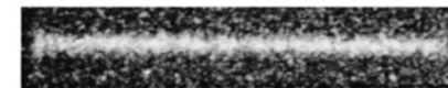
Fig. 1(b). Luminous image observed with the X-ray beam at 20 keV, corresponding to the photoelectron energy of 16.8 keV. The range of the photoelectrons was estimated to be 2.0 mm.
