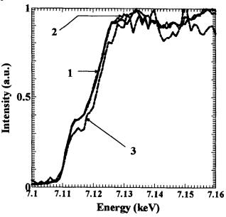
The spectra of iron in three different points in tissues around a retrieved implant. The curves 1 and 2 correspond to the points where the particles from stainless steel are dominantly present in the tissues, with high concentration. The curve 3 corresponds to a point with low concentration of metallic elements. The chemical state is remarkably different from that of Fe in stainless steel.
