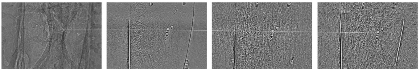
**Figure 3** Four particles of quarry dust are visible at the centre of the motion-detected frames. Particles did not aggregate or have the appearance of trapping liquid around them on the airway surface. In this sequence the quarry dust particles are moving at a rate of 0.41 mm/min.
