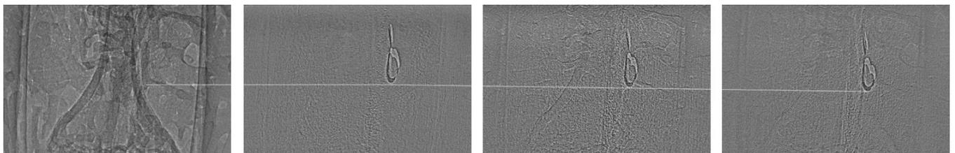
**Figure 4** Fibreglass appears similar to asbestos, but the objects were smaller and had shorter tails. Like asbestos, the fibres appeared to smoothly trap liquid around them so that individual fibreglass fibres could not be seen. Fibreglass moved at the same speed as the quarry dust, at 0.41 mm/min.
