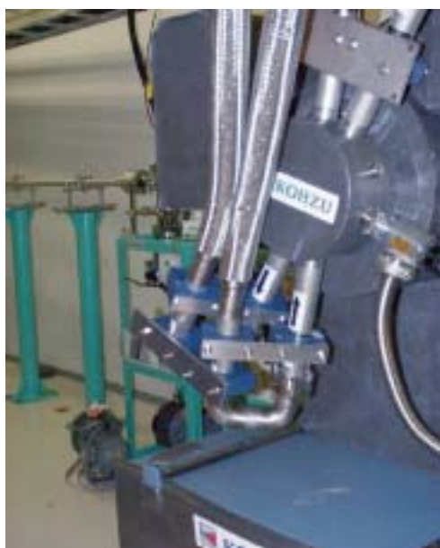
Fig . 6 The transfer tube of the circulating liquid nitrogen . The old tubes ( left panel ) were modified to the new one ( right panel ) to reduce mechanical vibrations .
