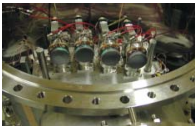
Figure 3 . Four analyzer crystal setup .
