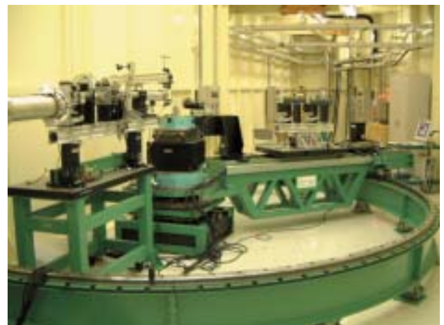
Figure 4 The IXS spectrometer installed in the experimental hutch of BL12XU , custom designed and manufactured by the Advanced Design Consulting , Inc .
