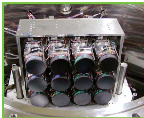
Fig. 1 Multi analyzer stage in the 10m vacuum chamber on the horizontal arm. Each analyzer has two degrees of motorized angular motion and a manual psi rotation, as well as temperature control stages.
