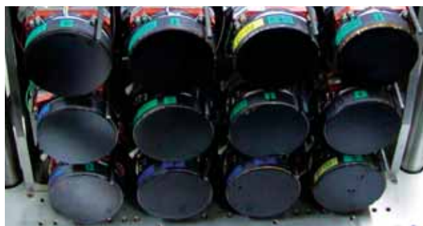
Fig.1 12 Analyzer array. Each crystal is about 10 cm in diameter.
