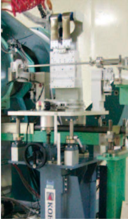
Fig.2 New IO Section including manual vertical translation and mounts for the KB setup and two slits (one in front and one behind)
