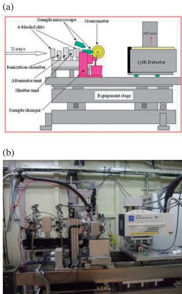
Fig.1 (a) Schematic and (b) real image of new protein end station.
