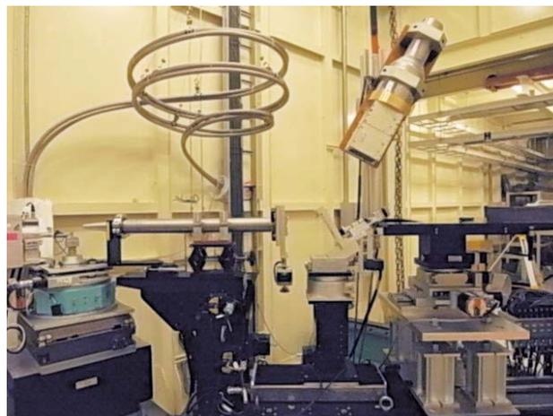
Fig.2 Bent-Laue spectrometer for IXS using 20 keV x-rays.
