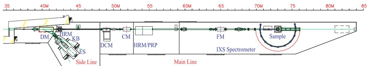
Fig.1 Schematic layout (top view) of the BL12XU: DCM a double crystal monochromator for the main line, CM a collimating mirror, HRM a high resolution (channel cut) monochromator, PRP a phase retarding plate, FM a focusing mirror, and IXS an inelastic X-ray scattering spectrometer. For the side line DM is a diamond monochromator, HRM a high resolution (channel cut) monochromator, KB a Kirkpatrick-Baez X-ray focusing (mirrors) system; ES stands for the HAXPES end station.
