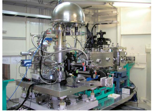
Fig.3 HAXPES End-station in the horizontal geometry (a), and the vertical geometry (b).
