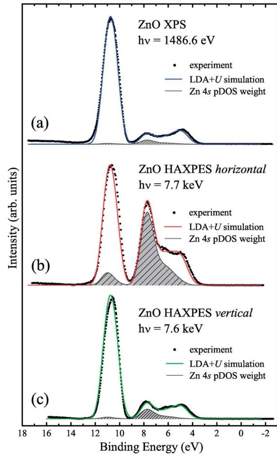
Fig.4 Photoemission spectra of ZnO detected using XPS source (a), 7.7 keV linearly polarized synchrotron source detected in the horizontal geometry (b), and 7.6 keV linearly polarized synchrotron source detected in the vertical geometry (c).
