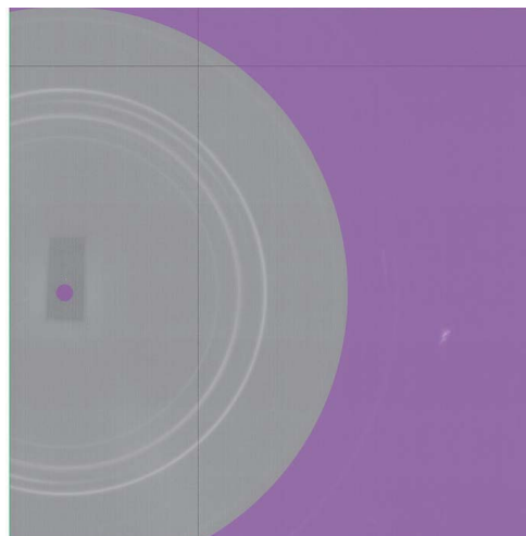
Figure 1. Powder pattern from an iron foil in a diamond anvil cell (DAC) at 53 GPa (work by Ohtani, et al. ). Rings are from the Re gasket and the Fe sample. Purple sections were not included in the analysis, and the grey patch at the center of the rings is the beam stop. Some care is required because the direct beam, with > 10 photons/sec is enough to damage the detector.
