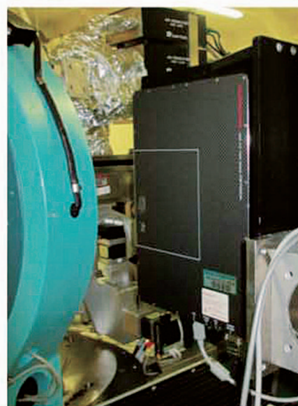
Figure 1. The upper panel shows the long focal length camera (right side) looking at the sample positions from a distance of about 1.5 m. It has a resolution of about 0.1 mm. The lower panel shows a photograph (from the opposite side of the spectrometer) of the area detector located behind the sample.
