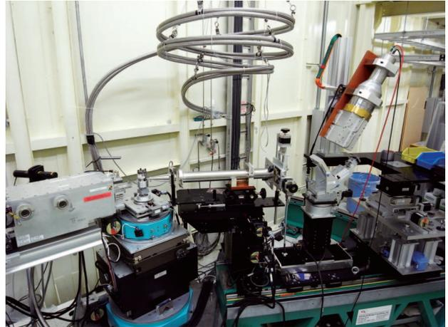
Fig. 2 FeS sample in diamond anvil cell, being measured by 20 keV spectrometer.
