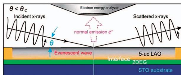
Fig. 4 Schematic geometry of photoelectron detection near normal emission with grazing incident x-rays near total external reflection.
