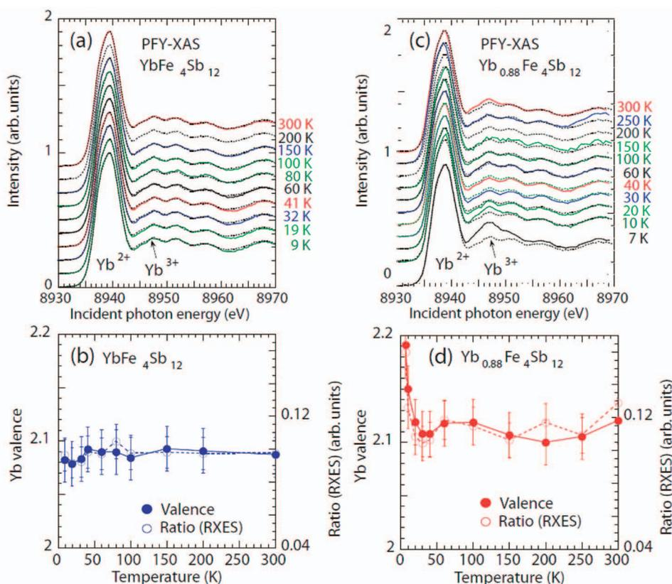
Fig. 3 PFY-XAS spectra (a) and derived valence number (b) of  $\text{YbFe}_4\text{Sb}_{12}$  while PFY-XAS spectra (c) and derived valence number (d) of  $\text{Yb}_{0.88}\text{Fe}_4\text{Sb}_{12}$  [Phys. Rev. Lett. **107**, (2011) 177203].
