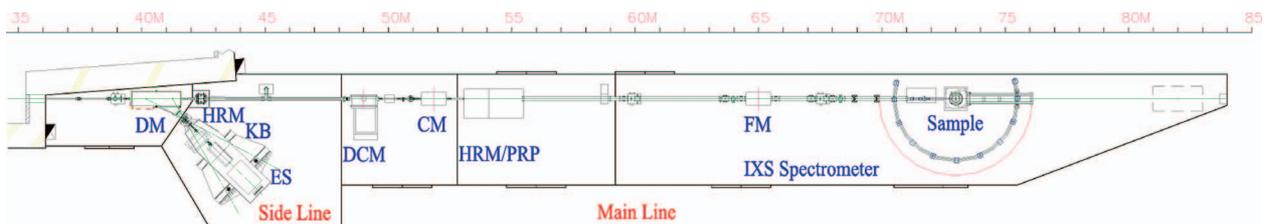
Fig. 1 Schematic diagram (top view) of the BL12XU: DM is a diamond monochromator for the sideline, DCM a double crystal monochromator for the mainline, CM a collimating mirror, HRM a high resolution (channel cut) monochromator, PRP a phase retarding plate, FM a focusing mirror, and IXS an inelastic x-ray scattering spectrometer.
