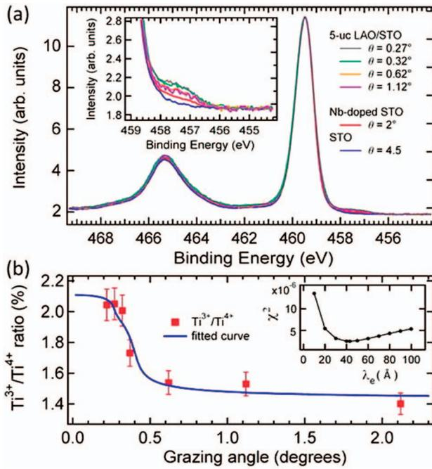
Fig. 5 (a) HAXPES spectra of Ti 2p with various grazing incident angles and samples. The inset shows enlarged region of Ti<sup>4+</sup>. (b) Measured ratios of Ti<sup>3+</sup>/Ti<sup>4+</sup> compared to a model fit.
