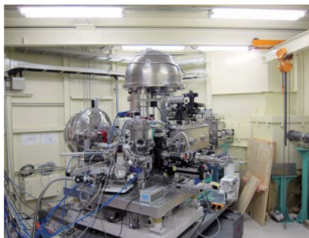
Fig. 4 Newly constructed HAXPES end station equipped with two electron energy analyzers for both horizontal and vertical geometries.
