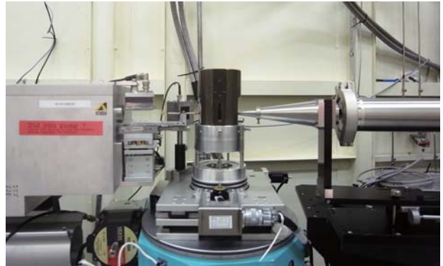
Fig. 2 Magnesium silicate mineral compressed in sintered-diamond anvil cell, mounted in the 20 keV bent Laue spectrometer.
