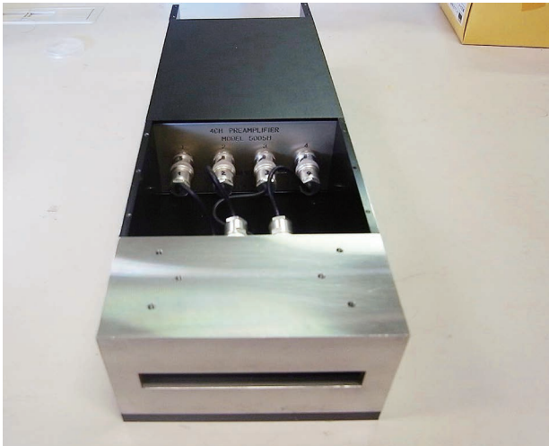
Fig.3 CdTe array detector (presently 4 elements, having 10 \times 10 \text{ mm}^2 each surface)
