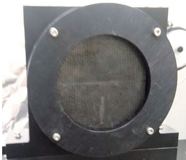
Fig.2 Photo of spherical quartz analyzer. Quartz itself is transparent but it looks black after bonded onto a substrate
