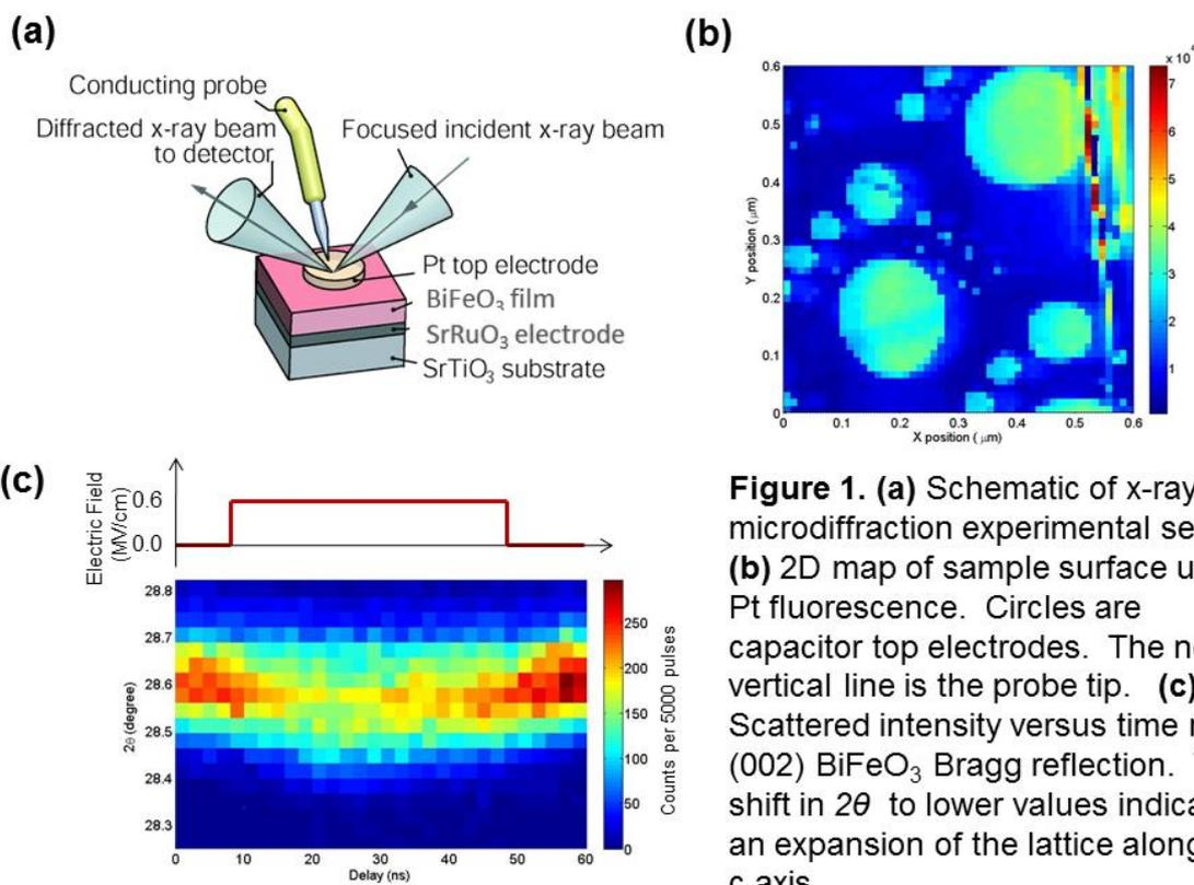
**Figure 1.** (a) Schematic of x-ray microdiffraction experimental setup. (b) 2D map of sample surface using Pt fluorescence. Circles are capacitor top electrodes. The nearly vertical line is the probe tip. (c) Scattered intensity versus time near (002) BiFeO<sub>3</sub> Bragg reflection. The shift in  $2\theta$  to lower values indicates an expansion of the lattice along the c axis.
