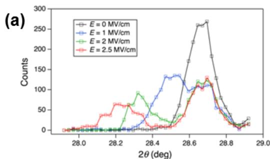
**Figure 2. (a)**  $\theta$ - $2\theta$  scans of (002) reflection at various electric fields. The unresponsive peak is at  $28.68^\circ$ , while the responsive peak position decreases as  $E$  increases.
