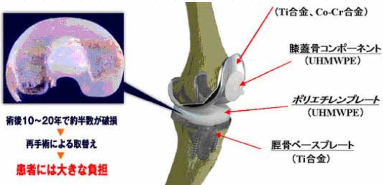
Fig1 . Structure of total knee prosthesis and damaged UHMWPE plate
