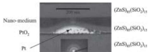
Fig. 1 TEM micrograph of a laser-induced bubble in the PtOx layer of a SuperRens disc.
