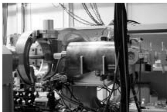
Fig.1 GI-SAXS chamber installed at BL13XU in the present experiment.
