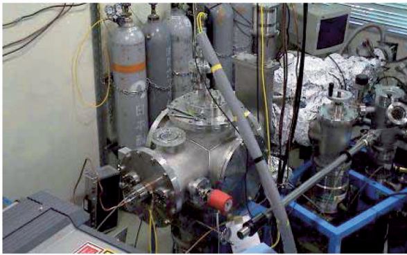
Figure 1 Laser-induced hyperthermal atom beam source at Kobe University
