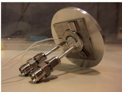
Fig. 2 The sample heating stage.
