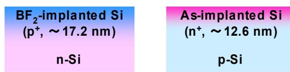
Fig. 1. Schematic of USJ samples.
