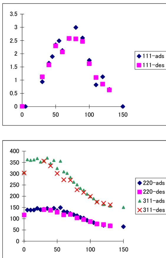
**Figure:** Absolute intensity of  $\text{N}_2/\text{AMS-8}$  as a function of pressure at 90K. (a)111 reflection. (b)220 and 311 reflections.
