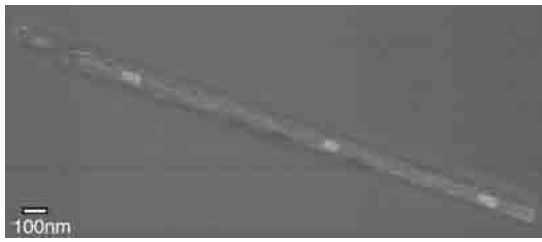
Fig. 2. TEM image of multi-segment nanowire \text{Ni}/[\text{Au}(50\text{nm})/\text{Ni}(1000\text{nm})]_2/\text{Au}(50\text{nm})/\text{Ni} .
