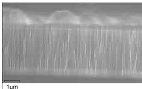
Fig. 1. Cross-sectional TEM image of self-assembled magnetic nanowire array in porous anodized aluminum template.
