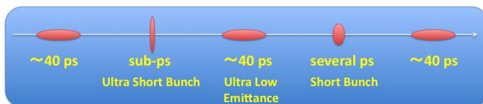
Figure 5.16: Short bunches are trapped in some specific buckets. Other buckets are dedicated for long bunches with the ultra low emittance.
