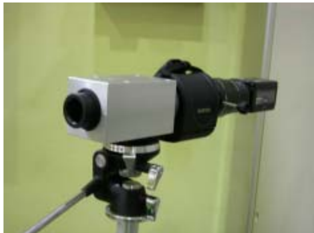
Figure 2: Spectrometer and I.I.-camera for the imaging spectrograph
