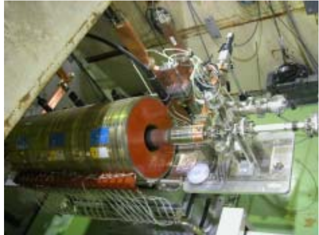
Figure 4: High-power test stand at KEK: The camera system is installed downstream to take spectrographs of light emitted due to rf breakdown.
